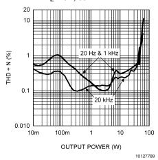
THD+N vs Frequency  $\pm$ 17V, f<sub>SW</sub> = 175kHz, P<sub>OUT</sub> = 1W & 50W R<sub>I</sub> =  $4\Omega$ , 30kHz BW
