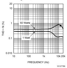
THD+N vs Frequency  $\pm 17V$ ,  $f_{SW}$  = 175kHz,  $P_{OUT}$  = 1W & 25W  $R_L$  =  $8\Omega$ , 30kHz BW
