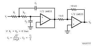
FIGURE 6. Pre-amplifier Stage with Low Pass Filter
