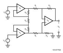
FIGURE 5. Feedback instrumentation Amplifier Schematic
