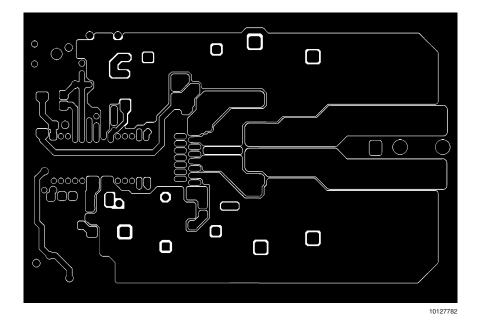
FIGURE 10. Reference PCB Top Layer
