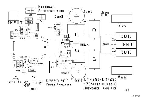
FIGURE 8. Reference PCB Silk Screen Layer
