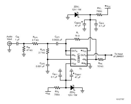
FIGURE 12. Input Pre-Amplifier And Filter Schematic
