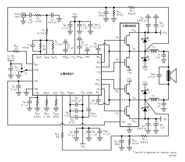
FIGURE 7. Reference PCB Schematic
