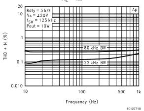
THD+N vs. Frequency vs. Bandwidth  ${\rm R_L} = 8\Omega$
