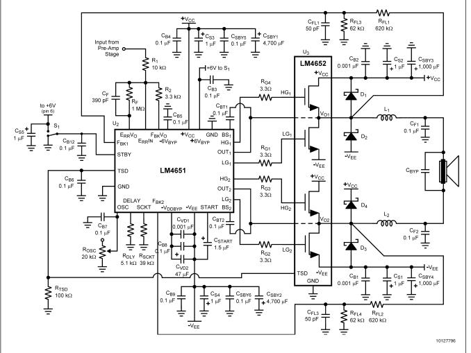
FIGURE 13. Full Audio Bandwidth Schematic
