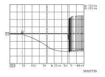
FIGURE 3. Startup Timing Diagram
