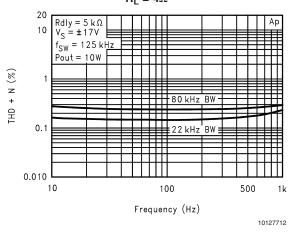
THD+N vs. Frequency vs. Bandwidth  $\mathbf{R_L} = \mathbf{8}\Omega$
