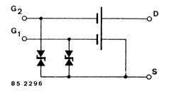
BF961 Marking Plastic case ( $\sim$  TO 50) 1 = Drain, 2 = Source, 3 = Gate 1, 4 = Gate 2 BF961 Marking Plastic case ( $\sim$  TO 50) 1 = Drain, 2 = Source, 3 = Gate 1, 4 = Gate 2
