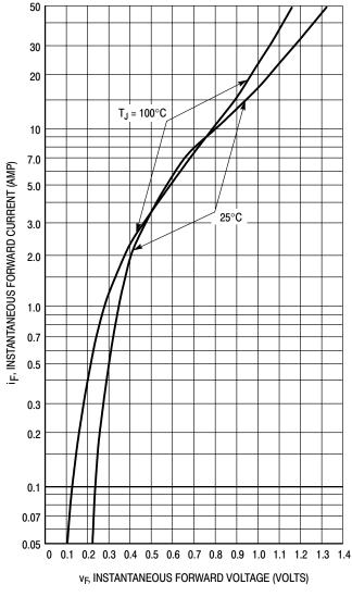
Figure 7. Typical Forward Voltage
