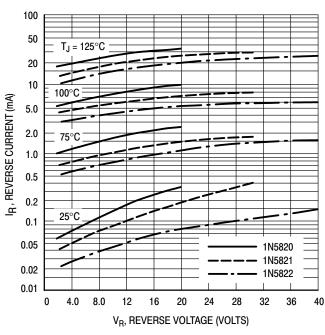
**Figure 9. Typical Reverse Current**
