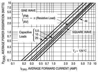
Figure 6. Forward Power Dissipation 1N5820-22
